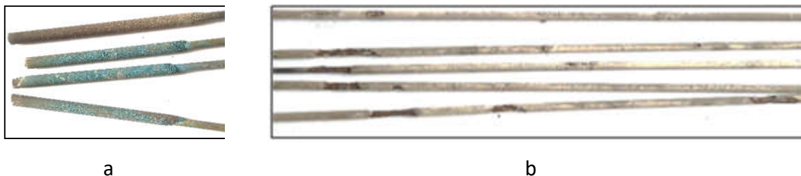
Figure 1. Waste welding electrodes: a – cinders; b – destroyed coating
