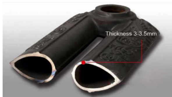
Fig. 1. Cast section of a household heating radiator
