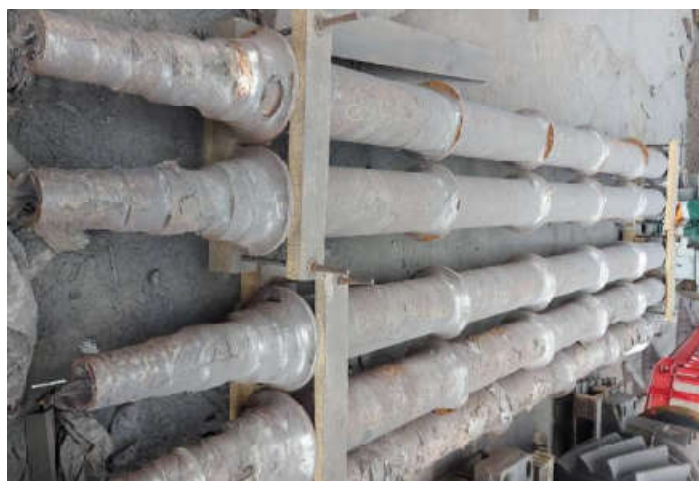
Figure 1 Shafts of the upper support of the pellet blasting furnace
