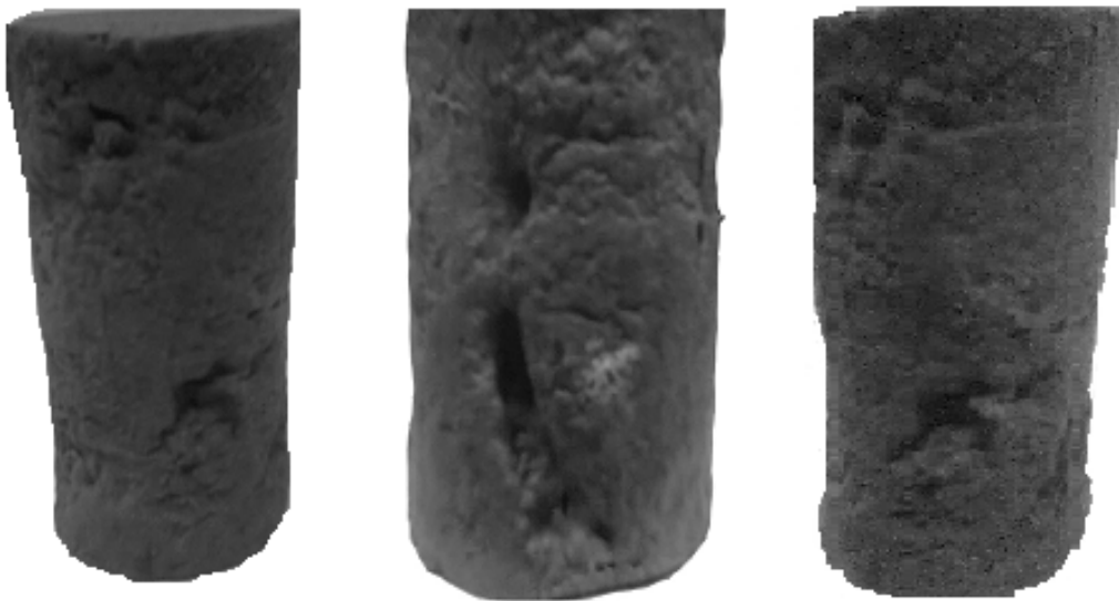
Figure 2 – Erosion in loess samples for filtration technique taking place in parallel with stratum
